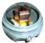
B - Earth Return Current units - Carbon brushes
