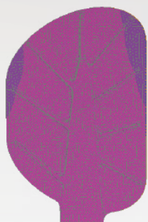
SiC optoSIC+ Deformation ± 0,32 μm
